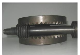
Fig. 4. Dual worm face gear with cylindrical pinion
