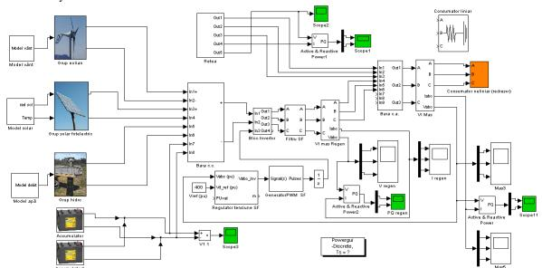
Fig. 3. Matlab/Simulink Simulation Model of a hybrid system based on renewable energy
