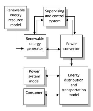
Fig. 2. Simulation Model Architecture based on RegenSim library
