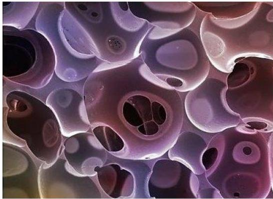
*Fig.2. Tempur memory foam polyurethane colored scanning electron micrograph magnification x264*
