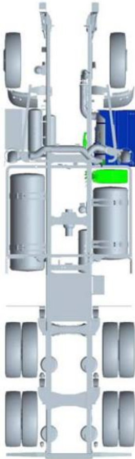
Figure 2: Catalyst integration on the vehicle chassis
