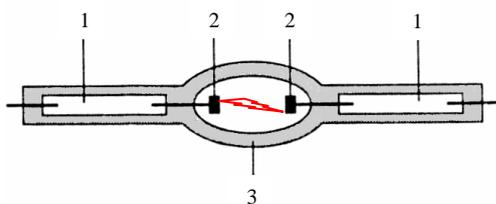
Fig. 1. Structure of gaseous discharge lamp (GDL)
