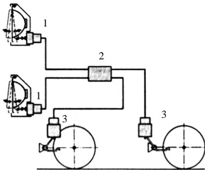
Fig. 5. Automatic vertical-aim control [1]
