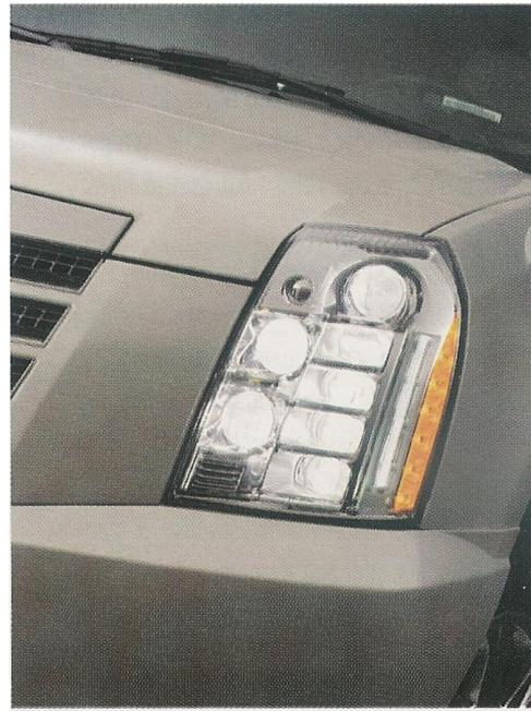
Fig. 13. The completely LED headlamp of Cadillac Escalade Platinum by Hella [4]
