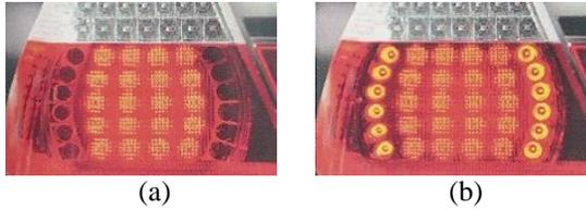
Fig. 9. Two level stop lamp [2]
