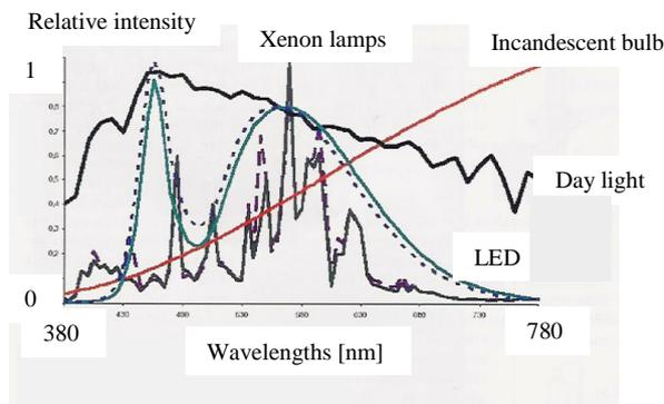
Fig. 16. Light spectrum for different lamps based on the work of Manz [3]
