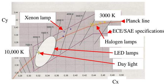
Fig. 15. Colour temperature of different lamps [2]
