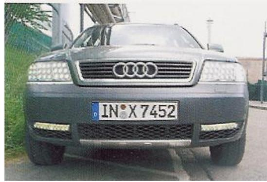
Fig. 12. Head lamp concept with LEDs [3]
