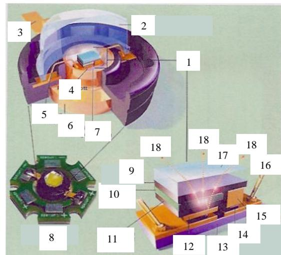
Fig. 7. Structure of LED applied at vehicles [2]
