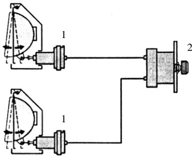
Fig. 4. Manual vertical-aim control [1]
