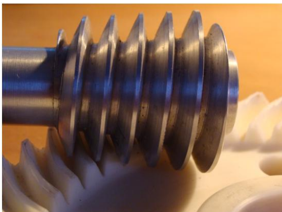
Fig. 1. The worm face-gear with reverse tapered pinion
