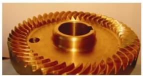
Fig. 3 The worm-wheel with reverse tapered
