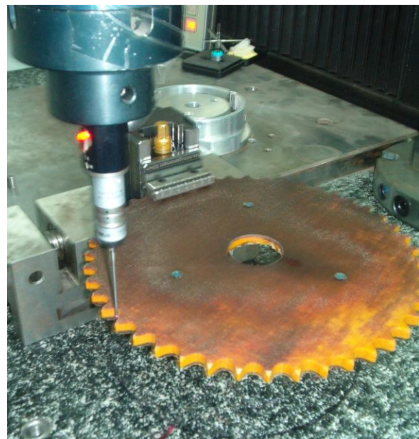
Fig. 12 - Frontal-radial aspect of measuring the chain wheel on "Smart CMM" [10]
