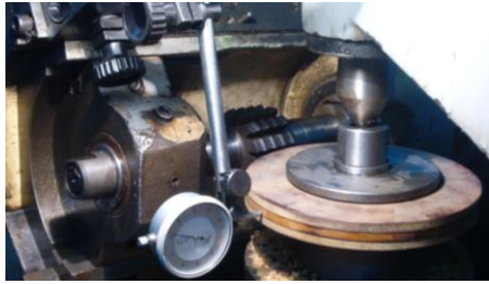
Fig. 3 - Checking axial beatings of sprockets semi-finished fixed for processing the teeth crown [7]
