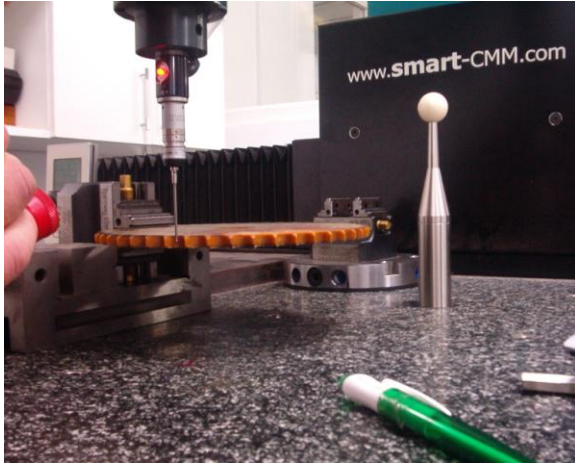
Fig. 13 - Axial aspect of measuring the chain wheel on "Smart CMM"[10]
