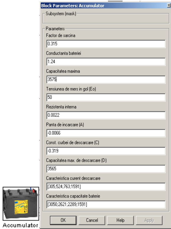
Fig. 7 – Accumulator block with electrical parameters input window
