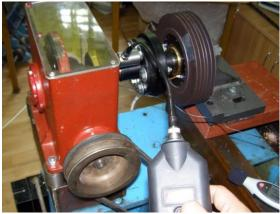
Figure 4 – Test gear box with test instrumentation
