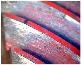
Figure 9 : Scratches was effective removed
