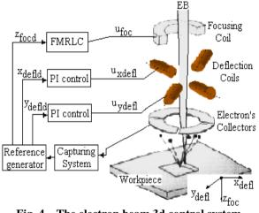
Fig. 4 – The electron beam 3d control system
