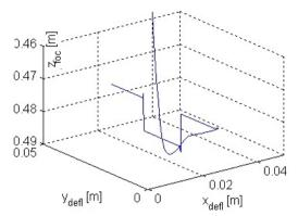
Fig. 7 – The 3D movement of the electron beam
