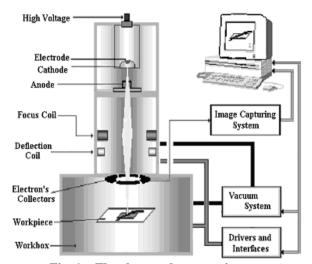
Fig. 1 – The electron beam equipment
