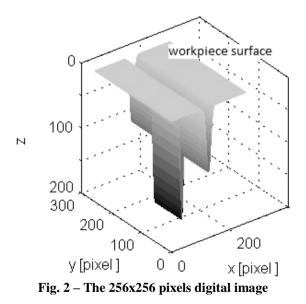
The desired 3D seam trajectory that must be extracted from the 256x256 pixels digital image is presented in Fig. 3. Also, the three-dimensional axes was converted to the real physical values [3,5].
