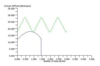
Fig.1 - Initial contact stiffness for considered gear transmission
