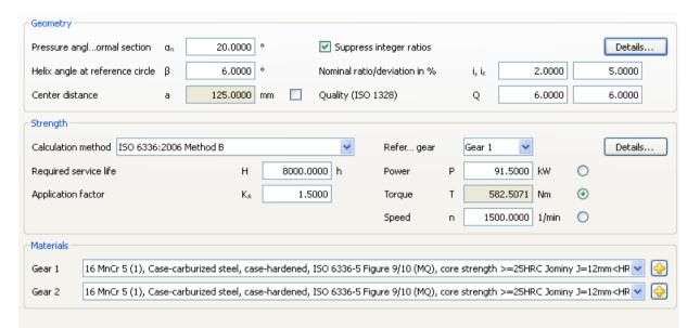
Fig. 2. Initial conditions for gears
