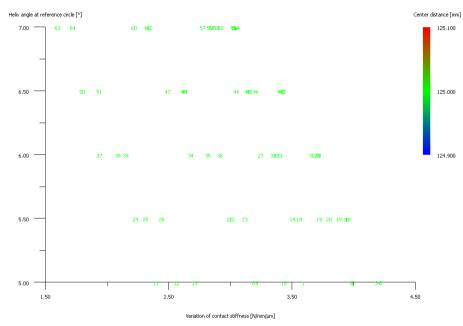
Fig.9. Variation of contact stiffness / helix angle
