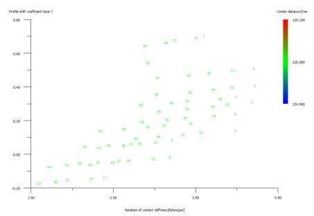
Fig.10. Variation of contact stiffness / profile shift coefficient
