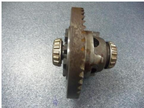
Fig. 5. Worm face gear differential
