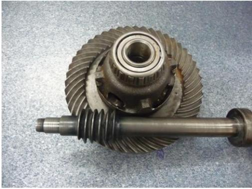
Fig.4. Worm face gear differential-view frontal
