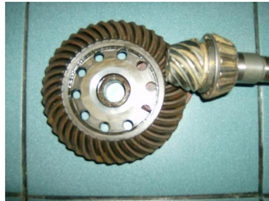
Fig.3. Hypoid pinion gear-wheel conical
