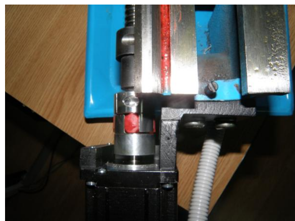
Fig. 2 -The mounting of the longitudinal motor and coupling
