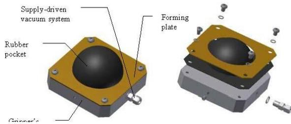
**Fig. 4** - The new gripper with granular material
