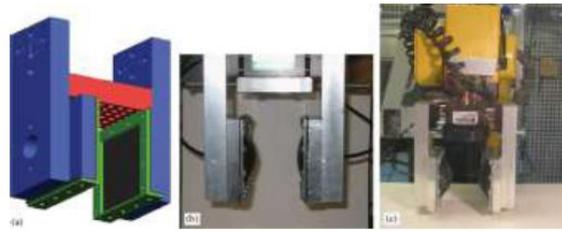
**Fig. 3** - Gripper used by Jiang et al. (a) selected conceptual model; (b) assembled gripper; (c) gripper attached to a robot
