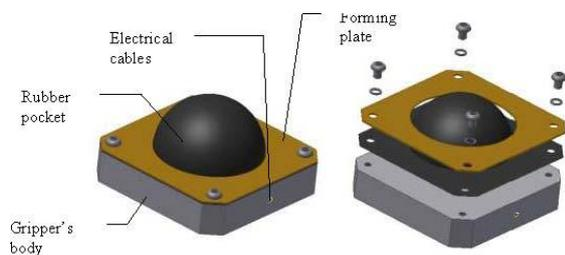
**Fig. 5** - The new gripper using the electrorheological fluid
