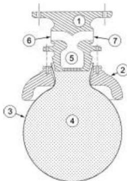
**Fig. 2** - Assembly drawing of the positive pressure jamming gripper, including components: 1) base, 2) external collar, 3) balloon membrane, 4) coffee grains, 5) air filter, 6) vacuum line port, and 7) high pressure port. The balloon is pinched between the base and the collar producing an airtight seal
