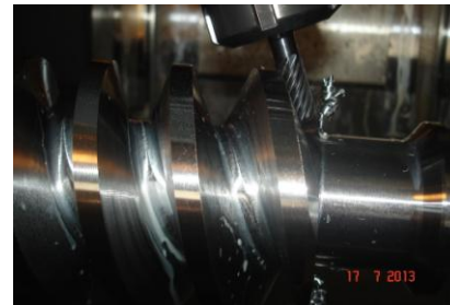
Fig. 4: Finishing right flank
