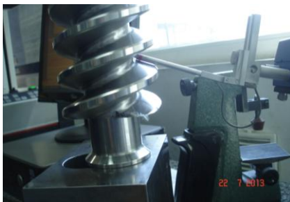
Fig.10. Roughness measurement along generators
