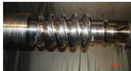
Fig. 5: The worm obtained after finishing
