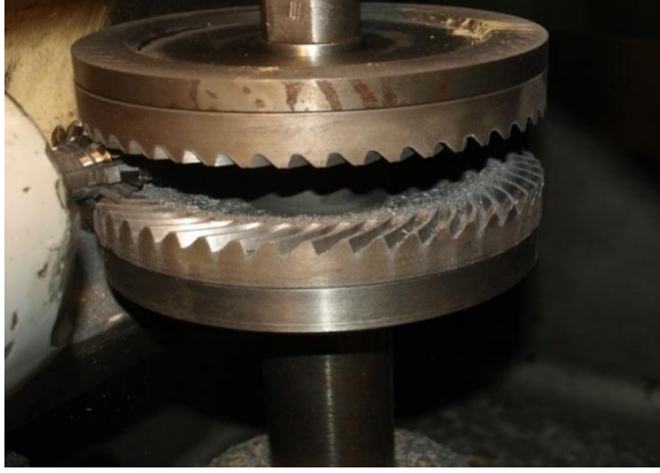
Fig. 1: Milling double worm-face wheel teeth through tangential advanced method with hob
