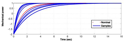
Fig. 3: The responses of an ideal turbine with  $T_{WS} = [0.5...6]$  sec. and  $T_{WS} = 2.75$  sec. as nominal value
