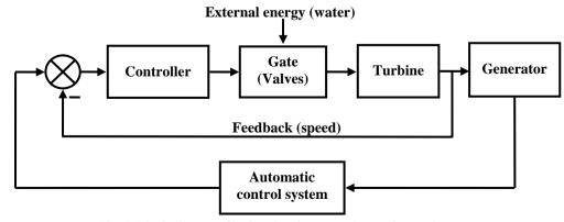
Fig. 5: Block diagram of hydro-electric power plant and control system
