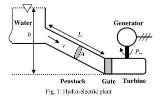
The dynamic behaviour of the hydro-electric plant depends, mainly, by: transient of water flow in water column; velocity (v) of water in the pipe with length
