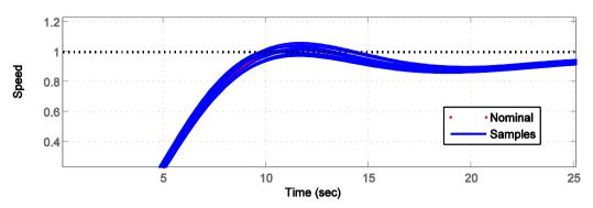
Fig. 9: The closed-loop response with:  $K_c = 1.250$ ,  $T_{WS} = 2.75 \pm 5\%$  sec.,  $T_l = 10 \pm 10\%$  sec.
