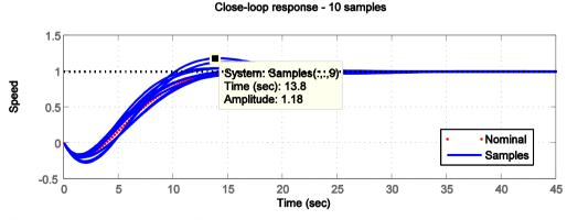
Fig. 8: The closed-loop response with:  $K_c = [1.136...1.388]$ ,  $T_{WS} = 2.75 \pm 20\%$  sec.,  $T_l = 10 \pm 20\%$  sec.
