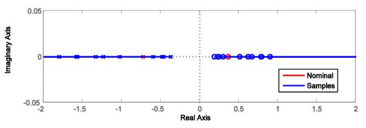
Fig. 2: Roots locus for of an ideal turbine with:  $T_{WS} = [0.5...6]$  sec. and  $T_{WS} = 2.75$  sec. as nominal value
