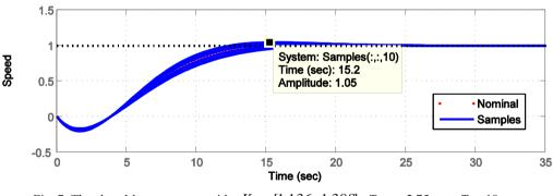
Fig. 7: The closed-loop response with:  $K_C = [1.136..1.388]$ ,  $T_{WS} = 2.75$  sec.,  $T_l = 10$  sec.
