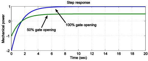
Fig. 4: The responses of an ideal turbine with  $T_{WS} = 2.75$  sec., to different gate opening
