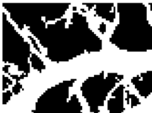
Fig. 5: Reference binary image imrefbwclean with salt&pepper noise removed
