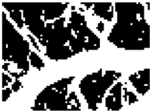
Fig. 4: Reference image transformed to binary image imrefbw presenting salt&pepper noise
