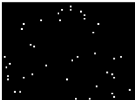
Fig. 9: Final image imramifications . Each little white square correspond to a ramification (see fig. 8). Number of resulted ramifications is 40
