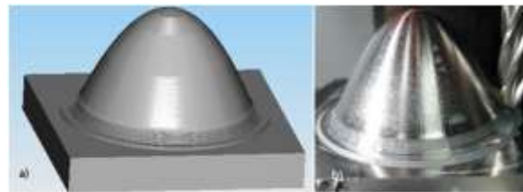
Fig. 5: An example of object based fragmentation: (a) CAD representation of the object defined by parabolic equation; (b) applying of the Spiral Milling Strategy to produce resultant surface finish
