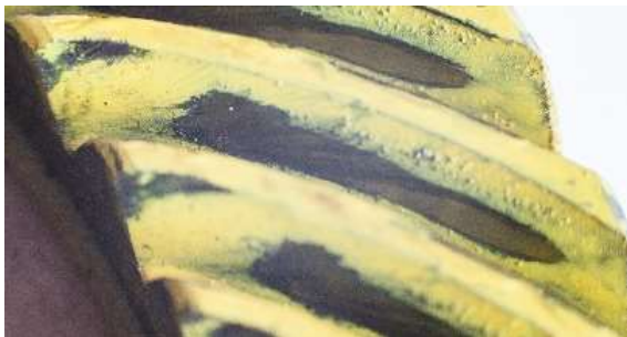
Fig. 8: Contact patch on the concave side gear in the combination of materials hardened steel / improved steel
