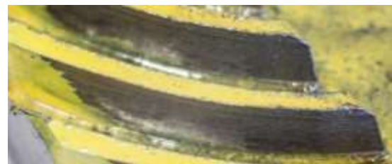
Fig. 5: Contact patch on the convex side gear in the combination of materials hardened steel/cast iron
