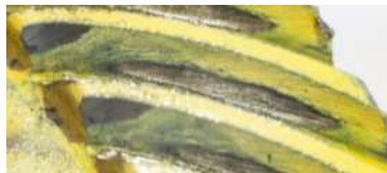
Fig. 6: Contact patch on the concave side gear in the combination of materials hardened steel / cast iron
