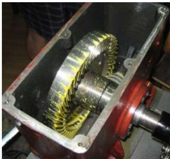
Fig. 4: Worm face gear with frontal speed reducer combination of materials hardened steel / steel improved
