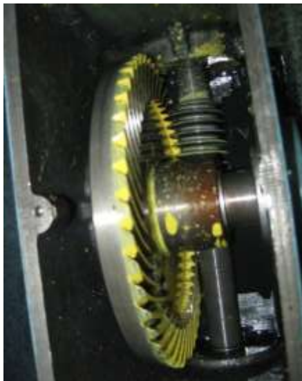
Fig. 3: Worm face gear with frontal speed reducer combination of materials hardened steel hardened / cast iron
