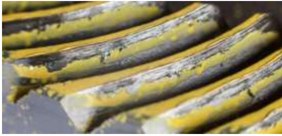
Fig. 7: Contact patch on the convex side gear in the combination of materials hardened steel / improved steel
