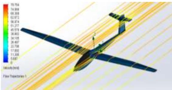
Fig. 10: Velocity distribution and flow trajectories around the sailplane
