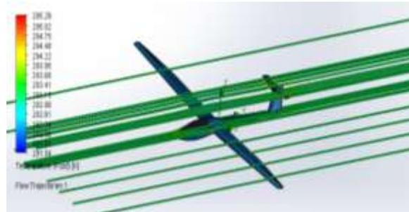
Fig. 11: The fluid temperature around the sailplane
