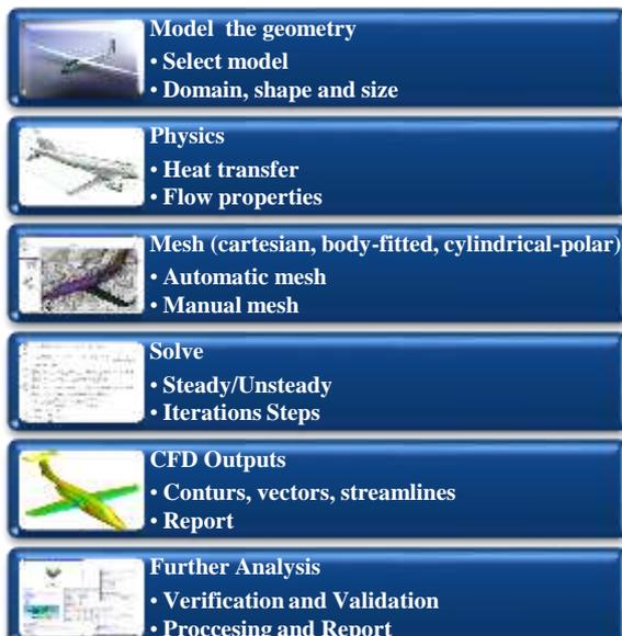
Fig. 5: CFD analysis process
