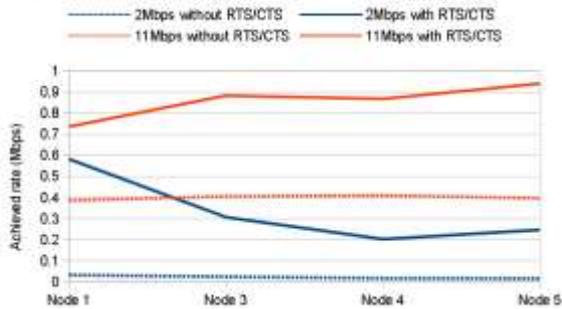
Fig. 5: Mean received rate, hidden terminal test, 5 nodes
