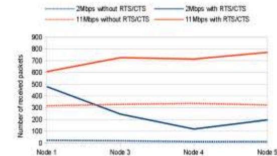
Fig. 3: Nr of received packets, hidden terminal test, 5 nodes
