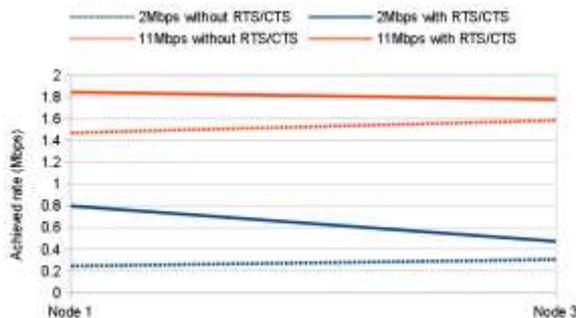
Fig. 4: Mean received rate, hidden terminal test, 3 nodes
