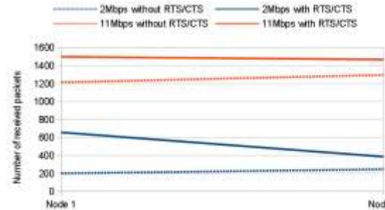
Fig. 2: Nr of received packets, hidden terminal test, 3 nodes
