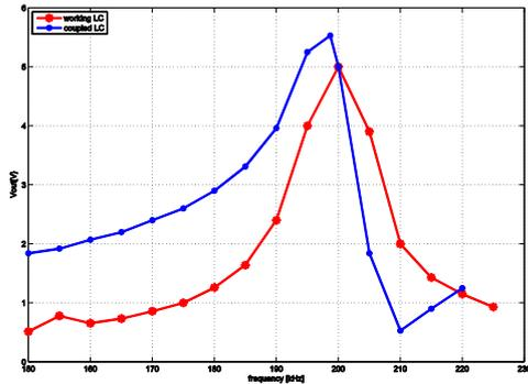
Fig. 5: The frequency characteristics of LC load
