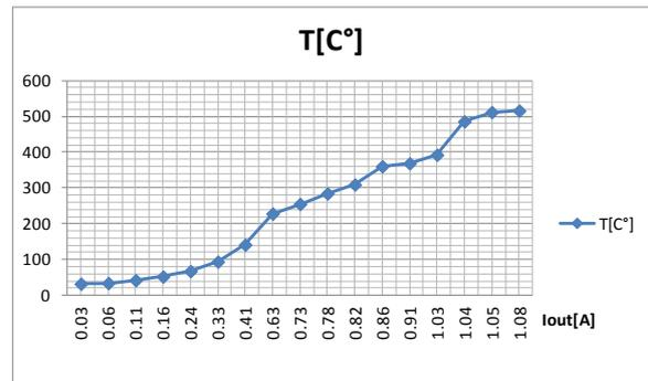
Fig. 8: The relationship between input current (from power supply) and obtained temperature
