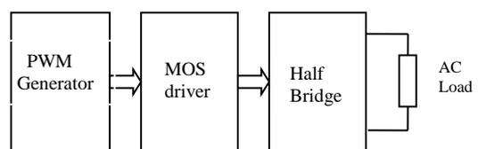
Fig. 4: The block schematics of the realized inverter
