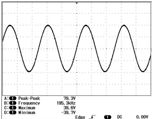
Fig. 6: The obtained inverters output signal
