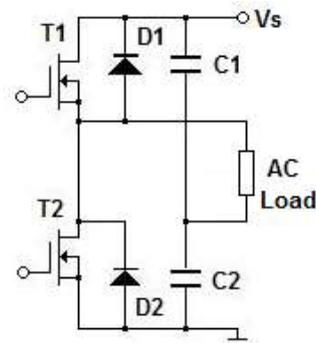
Fig. 2: The half-bridge inverter configuration
