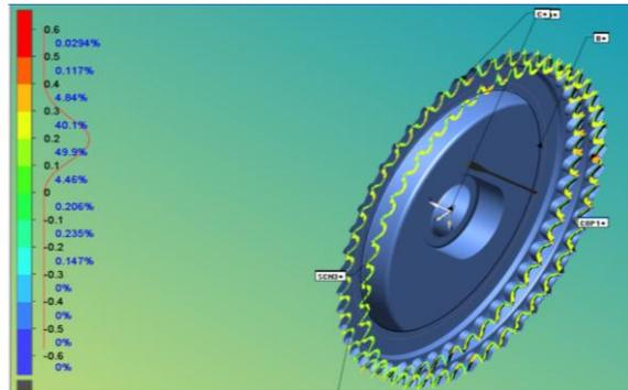
Fig. 20: - The graph of the profile deviation on the double toothing of the sprocket, in overall
