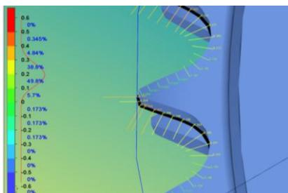
Fig. 18: The color graph of the scanning „SCN<sub>2</sub>” of the profile 1 of sprocket with double toothing
