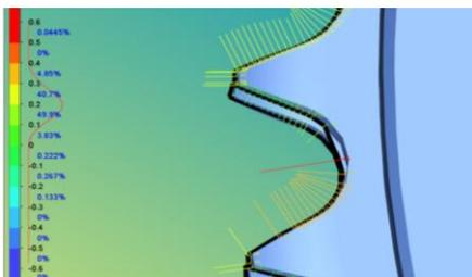
Fig. 19: The color graph of the scanning „SCN<sub>3</sub>” of the profile 2 of sprocket with double toothing
