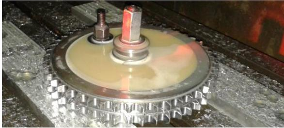
Fig. 11: Double tothing of sprocket in final stage of execution
