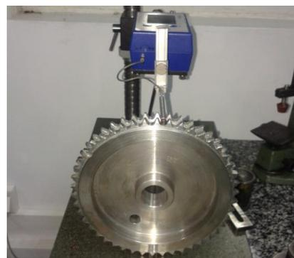
Fig. 21: Surtronic 25 – Portable and flexible surface finish measurement system [7]
