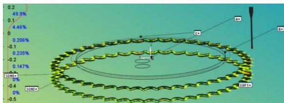
Fig. 16: The surfaces of the toothing profiles 1 and 2 scanned with „SCN<sub>2</sub>” respectively „SCN<sub>3</sub>” and the landmarks „A,B and C” corresponding to the surface of on sprocket with double toothing „PLN<sub>2</sub>”, circles „CIR<sub>3</sub>” and „CIR<sub>9</sub>”
