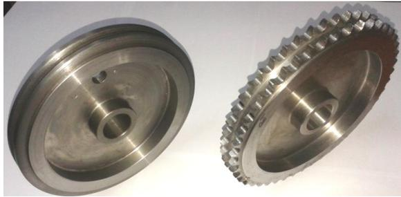
Fig. 12: The blank and the sprocket-completed
