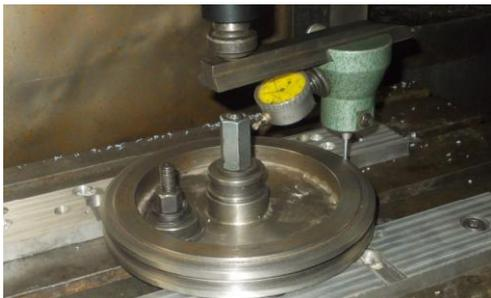
Fig. 5: Checking with the comparator clock of the precision of fixing the blank on the mass of „AXA” center
