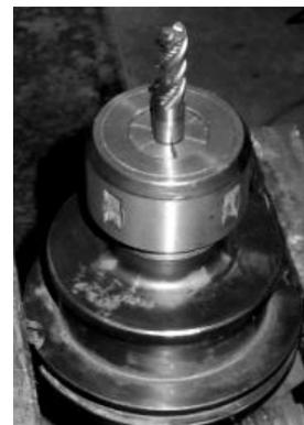
Fig. 3: End mill characteristics used at machining of the profile are  $\phi = 8$  [mm] and  $z = 4$  [teeth]
