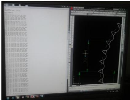
Fig. 4: Introduction of G codes in processing program, simultaneously with determining points on toothing profile
