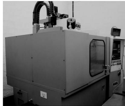
Fig. 1: „AXA VSC 0-500M” Controlled Vertical Machining Center [2]
