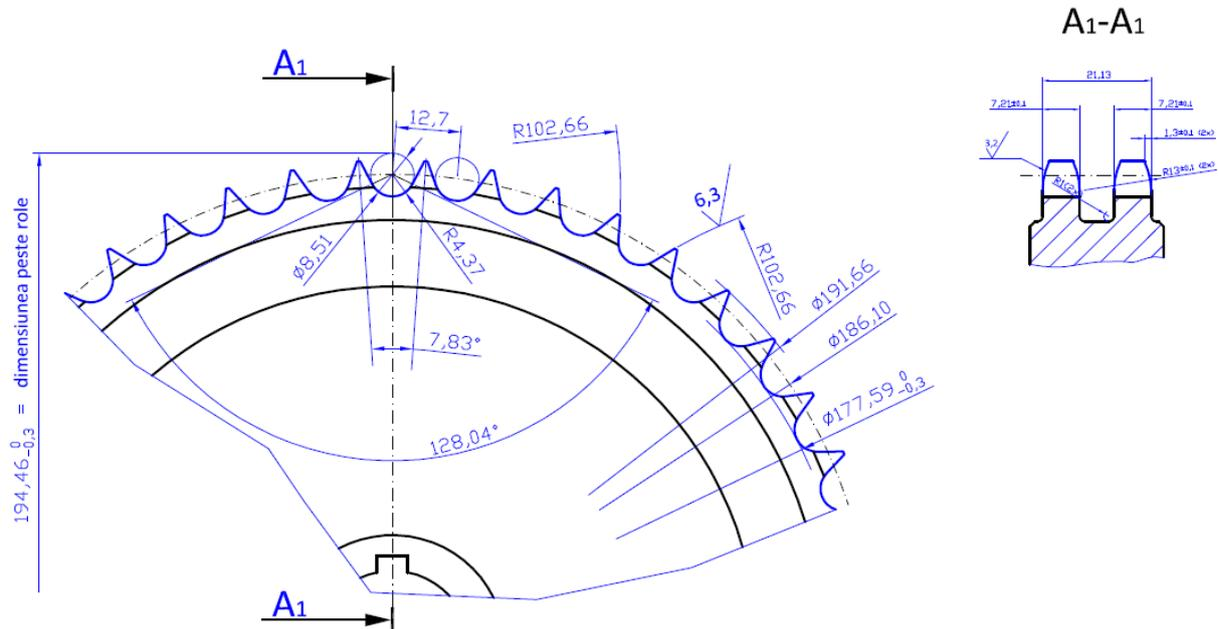
Fig. 2: Double profile of studied sprocket
