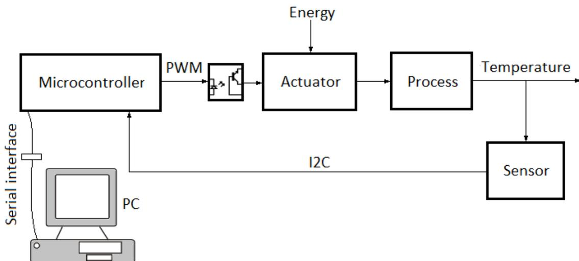
Fig. 1: The block diagram of the temperature control
