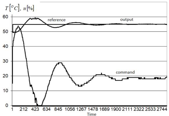
Fig. 8: PI control with set point of 55°C
