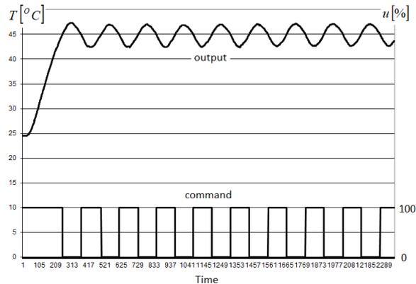
Fig. 6: On-off control with set point of 45°C
