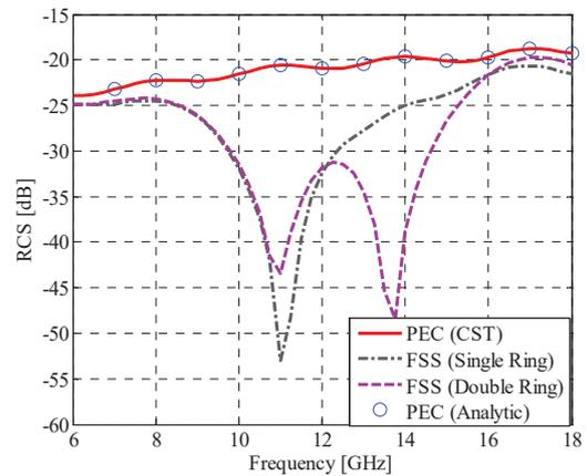
Fig. 3: Simulated monostatic RCS of the proposed single and dual-band cylindrical absorbers.
