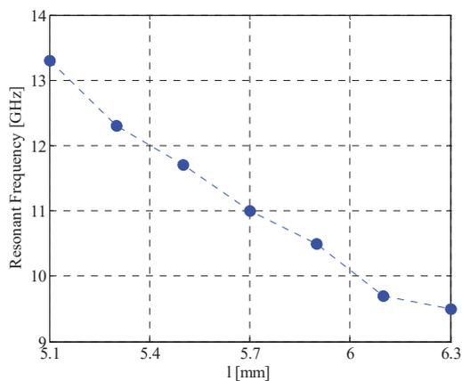
Fig. 5: The variations of resonant frequency of single band cylindrical absorber with parameter  $l$ .
