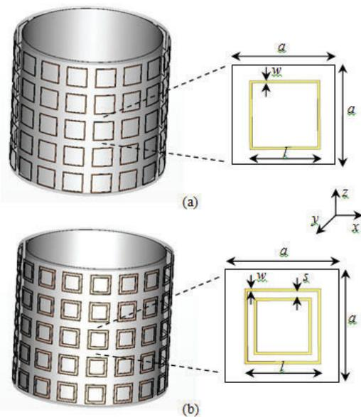
Fig. 1: The Geometry of (a) single band, and (b) dual-band cylindrical absorber structure. ( $a = 8$ mm,  $l = 5.7$  mm,  $w = 0.2$
