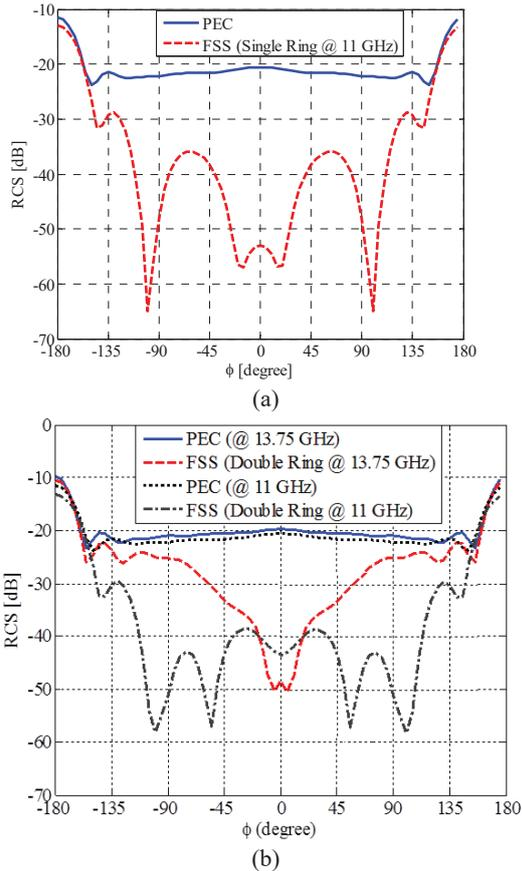
Fig. 4: Bistatic RCS of coated PEC cylinder at the resonant frequencies of (a) single band, and (b) dual-band absorbers.
