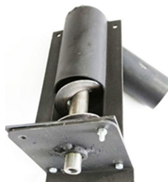
Fig. 4: Auger with feeding tube [22]
