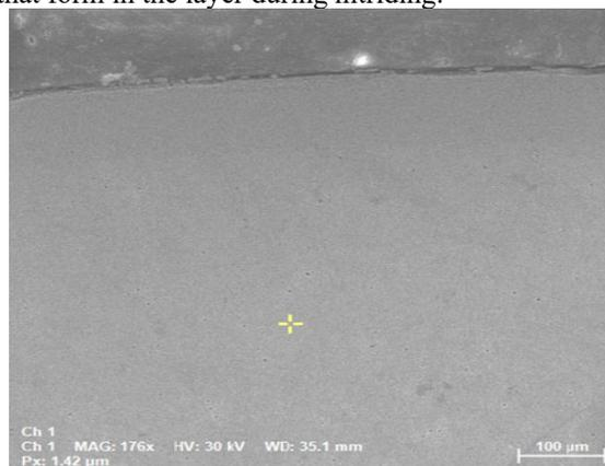
Fig. 9. SEM images of the 40Cr130 sample core, quenched from 1040°C, tempered to 510°C and nitrated at 520°C.
