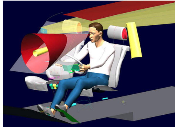
Fig. 7: Model in the ergonomic testing of the passenger compartment for the driver of the vehicle [14]
